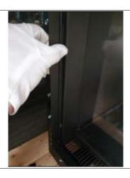
Step 4: For models with the side  $glass \, remove \, the \, outer \, rear \, side$ trim. Grip the trim and apply an upwardmotiontodisengagethe securing tabs from the slots in theinnertrim. When the tabsare clear of the slots. For model GF3 remove the outer trimboth sides.
