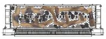
$\label{lem:eq:condition} Evenly place the remaining Embers around the Grate$ area, but avoiding the Burner tubes, as shown.
