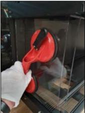
Step 5: For models with the side glass. With the outer front glass panel and trims removed. With one hand holding the glass pad, with an upward motion lift the top of the glass until engaging with the top of the inner fascia. The bottom of the glass is now clear of the bottom supporting channel. Swing the bottom of the glass outward with one hand holding the glass pad andtheotherhandgrippingthebottomcentreedgeof the glass. Remove the glass panel and retain in a safe place.
