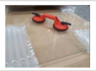
Step 2: Remove the outer glass panel from the bubblewrap. Laytheglass downhorizontally on the supporting surface and apply the glass suction pad (provided) to the centre of the glass and engage.
