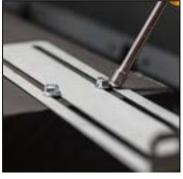
Step 3: To adjust the side spacer/s slacken thetwoboltsretaining the side spacers. Adjust the side spacers to the length to maintain the desired clearance 250 mm.
