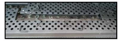
Place fibre embers only on the burner crosslighting ports by avoiding the main slotted port.
