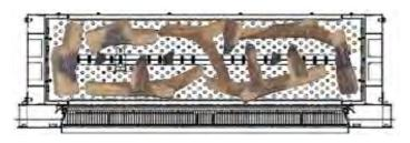
STEP 12  $Place \ 3 \ Embers \ on \ top \ of \ the \ Burner Tubes \ as \ shown.$
