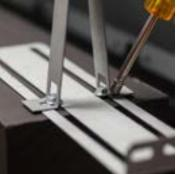
Step 2: With the top spacer in the vertical position insert the bottom flange of the top spacer onto the slackened off bolt head and tighten. Repeat so there are 2 x rear spacers and 2 x top spacers in position.
