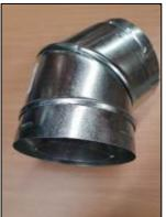
Elbows and bends create resistance within the venting configuration, and they must be included when determining the minimum and maximum fluing lengths. There must be an absolute minimum vertical rise of 600 mm before any elbow but preferably a vertical rise of 900 mm is recommended. Maintain the maximum length of straightflue between elbows or bends.
