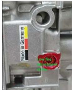
When the pressure register's thew pressure as nominated pages 10-14 turn to high fire and check the high fire has not deviated from burner pressure on High as nominated pages 10-14. Disconnect the manometer from the inlet pressure point and tighten the screw
