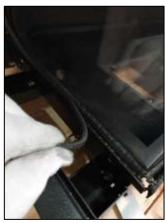
Step 2: The inner side glass is secured into the top, side and inner bottom supporting channel by rope seal. Grip the front edge of the rope and applyupwardmotiontoremovetheropefromthe channel.
